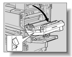
**2** Lift up the inside cover M4, and the pull out any misfed paper.
